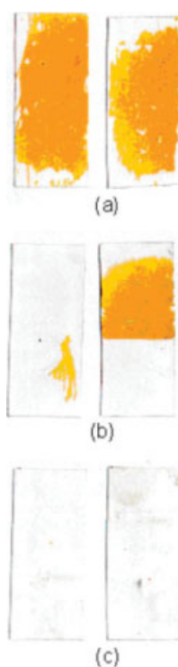
Figure 5 Photographs of the adhesive tapes after pull from a-C:H films deposited onto a PET surface without treatment (a) and with oxygen plasma treatment for (b) 1.5 and (c) 2.5 min. [Color figure can be viewed in the online issue, which is available at www.interscience.wiley.com .]
